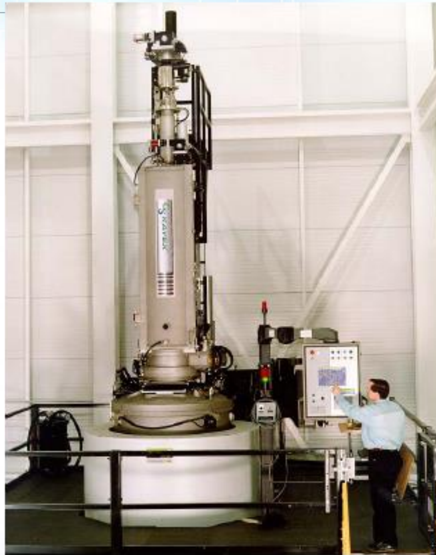
Photograph courtesy of Kayex Corp., 300 mm Si crystal puller
