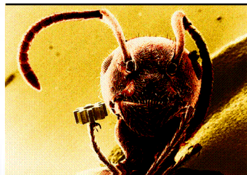
Nickel structure of an electrostatic linear actuator after electroforming and dissolution of the remaining resist parts. The structure height is 80 \mu\text{m} .
