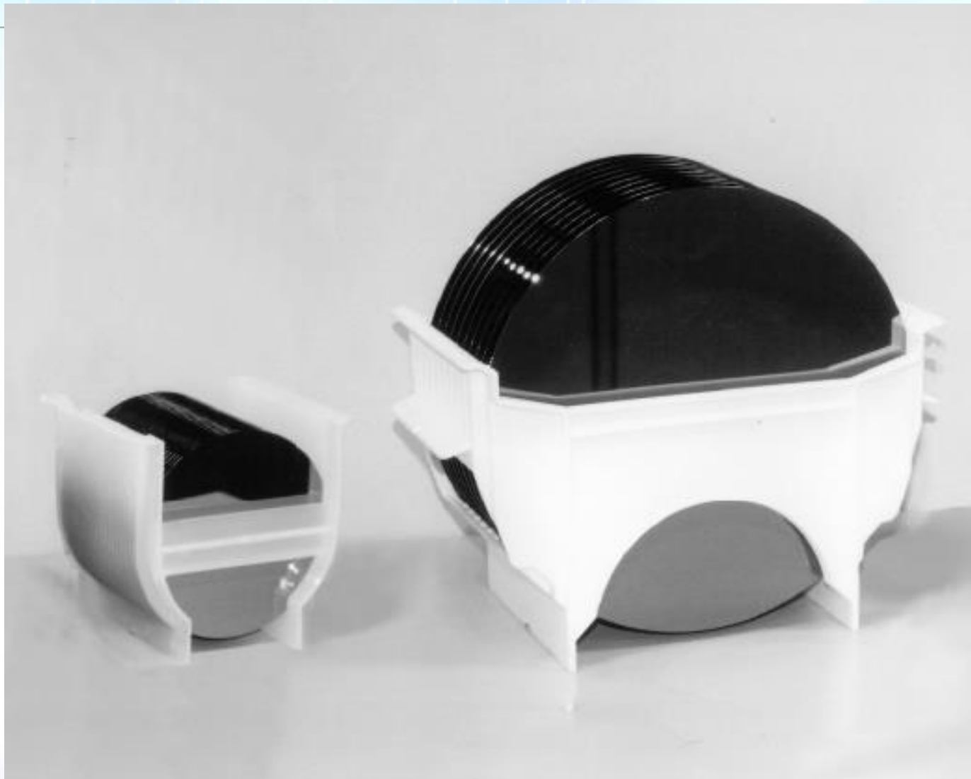
200-mm (8 in.) and 400-mm (16 in.) polished silicon wafers in cassettes.
